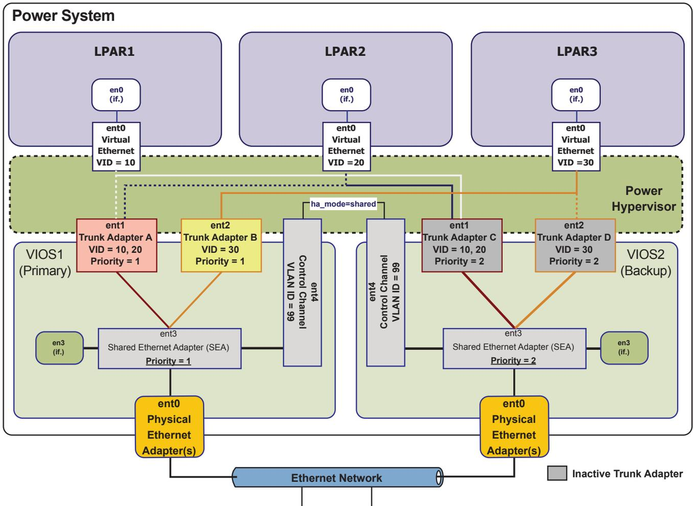
Figure 3: Shared Ethernet Adapter Failover with Load Sharing
